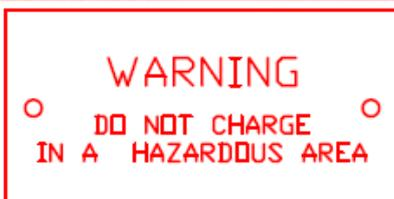
Warning label fitted when equipment is not supplied with an approved charger
