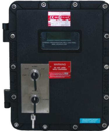
The CPFG-4000 is a PLC based Combined Pressurisation Fire & Gas control panel used in conjunction with other JCE supplied products such as gas /smoke detectors & pressure switches. A complete pressurisation control system can be constructed to monitor the conditions within pressurised modules used in areas which are potentially hazardous by the presence of flammable liquids, gases, or vapours.
