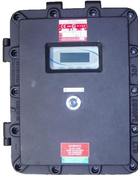
The MFGP series is a PLC based Fire & Gas control panel. Used in conjunction with other JCE supplied products such as gas/smoke detectors, these systems, and variations of it can be utilised to monitor the conditions of fire or gas in the atmosphere. The MFGP series is capable of monitoring signals from a single fire channel and three gas channels simultaneously. It is suitable for use with either Pellistor type or Infrared gas detectors, as standard.
